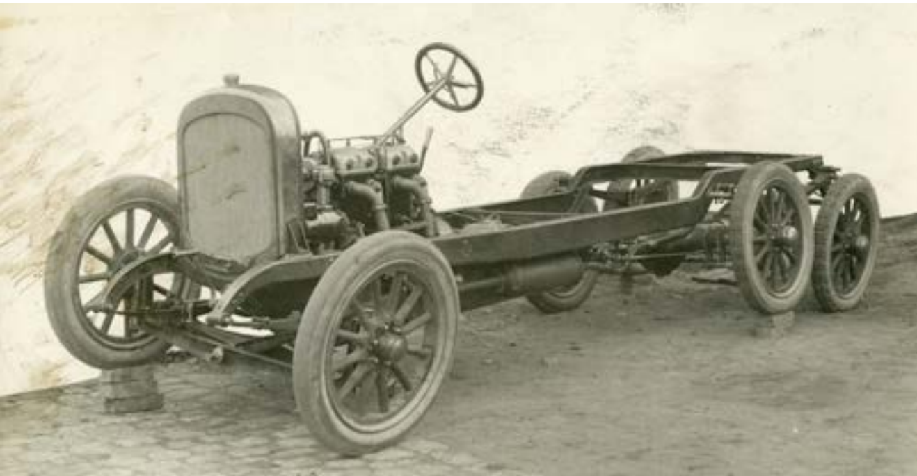
A picture of Mustad's car under construction in 1917. The chassis was built in the workshop of Mustad og Søn, and then fitted with a body built by O. Sørensen's Værksteder. (Photo: H Brinchmann, Kristiania)
