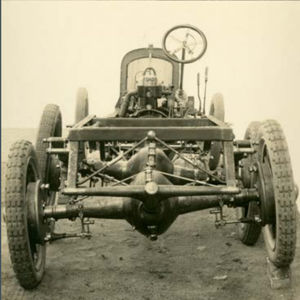
This photo of the complete chassis before the bodywork was mounted in 1917 shows the patented structure with suspension that allows the rear axles to move independently of each other. At the top: A drive with the family in an open car (Photo from the Mustad family)
