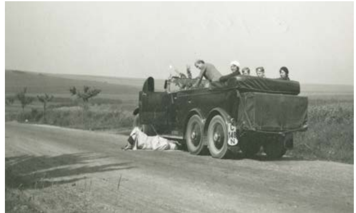
This picture is probably of one of the daughters checking that a lifting cylinder is back in place after a puncture. Here the car has the steel rims that were added in the 1927 alteration, but it is still open. The folded hood was attached at the rear, to carry the luggage the family would bring on their trips at home and abroad.
