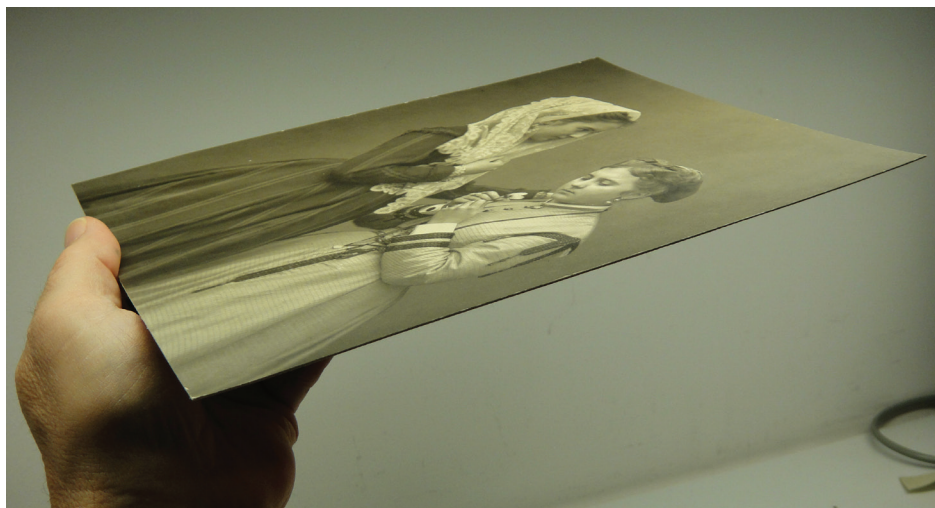
Figure 9 Viewing direction of about 180 degrees during visual identification of a carbon print.
